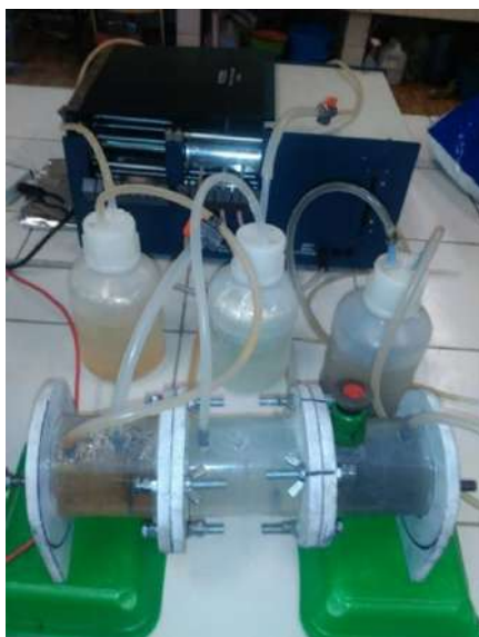
Figure 28. Photograph of the laboratory-scale three-chamber bioelectrochemical system operating as a microbial desalination cell (MDC).
