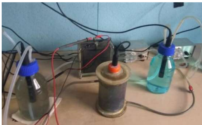
Figure 26. Photograph of the sandwich-type bioelectrochemical system used in Variant 2.
