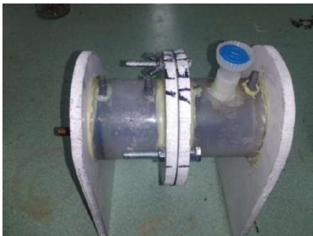
Figure 24. Photograph of the microbial fuel cell used in Variant 1.
